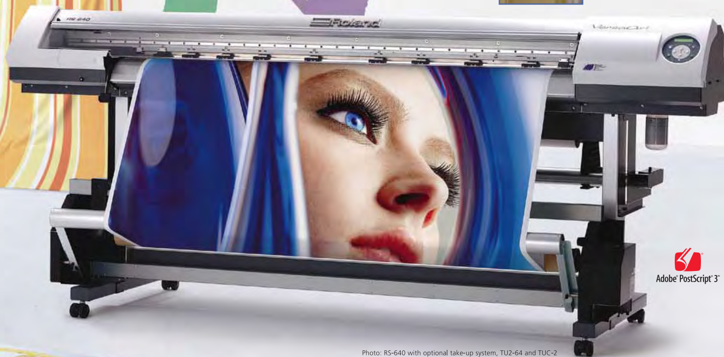
Photo: RS-640 with optional take-up system, TU2-64 and TUC-2
